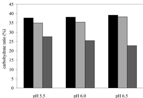
**Figure 3.** Effect of the pH value on the hydrolysis of lactose and product formation when using an initial lactose concentration of 10% (reaction conditions: 40°C, 24 h reaction time,  $\beta$ -galactosidase activity 2.5 U/mL). Sugars are given as the percentage of total sugar content in the mixture. ■, Glu; ■, Gal; ■, GalOS.
