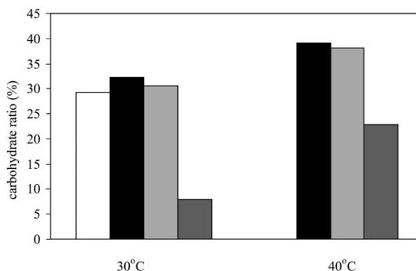
**Figure 4.** Effect of temperature on the hydrolysis of lactose and product formation when using the initial lactose concentration 10% (reaction conditions: pH 6.5, 24 h reaction time,  $\beta$ -galactosidase activity 2.5 U/mL). Sugars are given as the percentage of total sugar content in the mixture. □, Lac; ■, Glu; ■, Gal; ■, GalOS.
