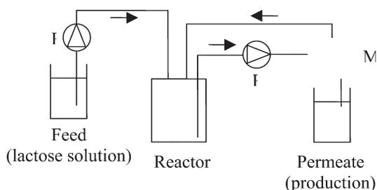
**Figure 1.** Scheme of the continuous laboratory scale reactor with an external crossflow ultrafiltration unit. P, peristaltic pump; M, UF membrane.
