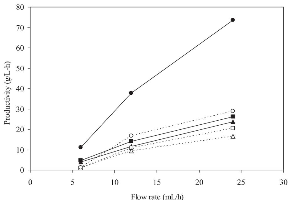
**Figure 7.** Formation of GalOS in a continuous reactor: Effect of both the substrate concentration and flow rate on the productivity; GalOS (circles), Glu (squares) and Gal (triangles). Experiments were carried out using an initial lactose concentration of 10% (opened symbols) and 20% (closed symbols).
