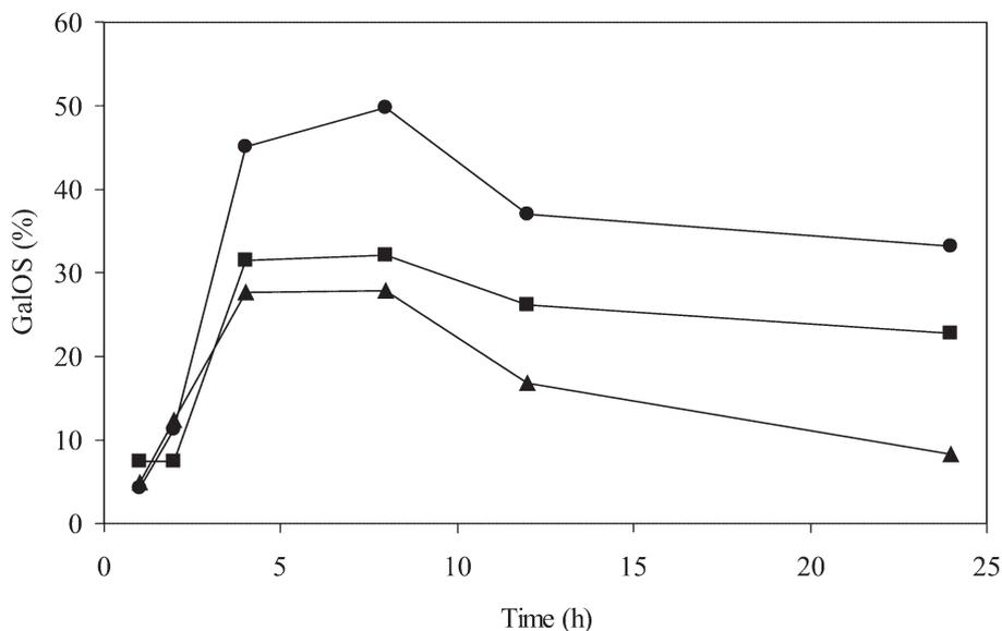
**Figure 5.** Time course of lactose hydrolysis in enzymatic batch reaction when using different initial concentrations of lactose: (▲) 5%, (■) 10% and (●) 20% (reaction conditions: 40°C, pH 6.5;  $\beta$ -galactosidase activity 2.5 U/mL).
